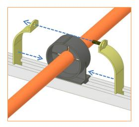
4. Thread locknut on stud and secure. Stud torque specification available upon request.
